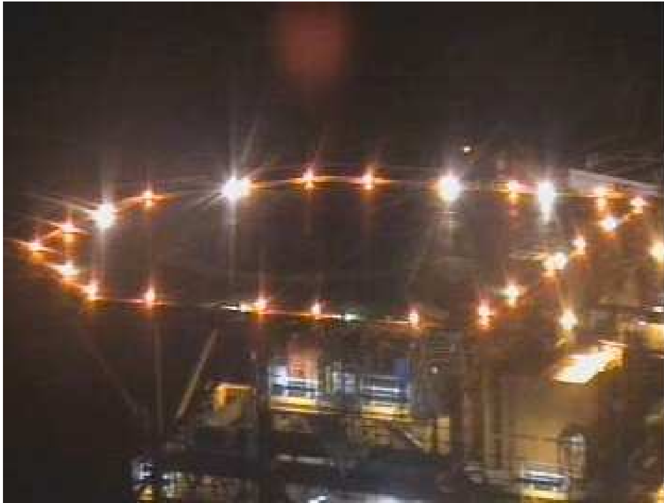
11.1 Figure 1: Example of Glare on a Helideck
